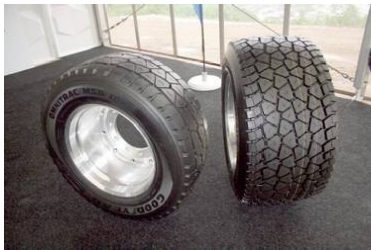
Industry first 385/55 R22.5 MSD II and 495/45 R22.5 MSD Mixed Service Super Single drive tires
