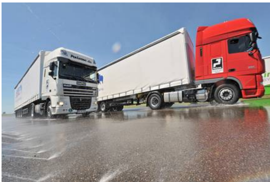
Wet braking difference – the red truck does not have LHT II
